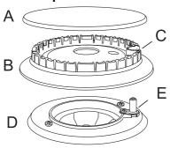
A cap, B head, C notch, D base, E electrode
